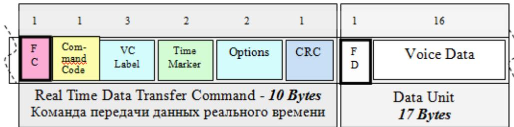
Figure 3b). Virtual channel voice traffic transfer.
